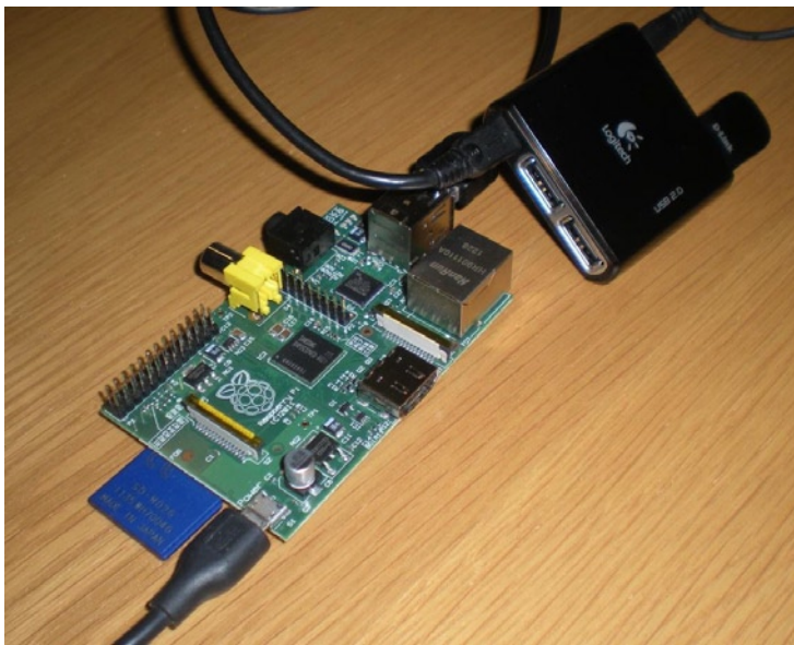
Figure 9-12. Powered USB hub in action
